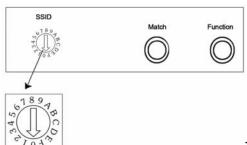
The dial code is used for setting WiFi-LED controller Ssid number,
