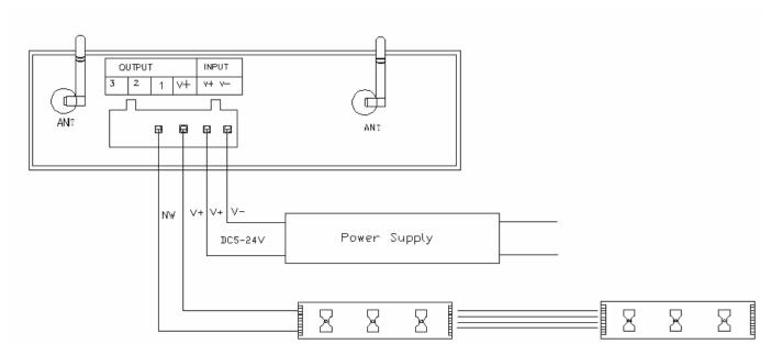
When connect three channels LED, you should put the Magic Color 1.0 software switch to DIM mode to use, under this mode, use color disk control the LED's brightness, Adjust process can be seen in the upper left corner NM numerical with change.
