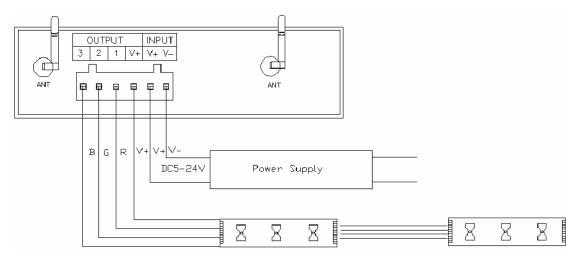
When connect three channels LED, you should put the Magic Color 1.0 software switch to CD mode to use, only under this mode, you can control the LED's color, brightness and speed. Color disk adjust the color (Adjust process can be seen in the upper left corner R, G, B numerical with change), speed/brightness item adjust speed and bright ("M"set the LED dynamic effect, "M"adjust the LED dynamic change.
