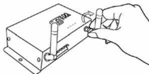
ANT's installation drawing: clockwise install WIFI antenna and anticlockwise take down the antenna.
