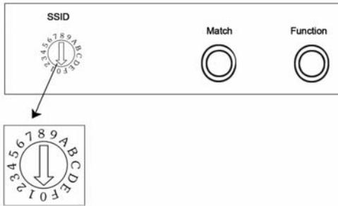
The dial code is used for setting WiFi-LED controller Ssid number, corresponding table as below. Form 0 to F, have 16 code in total, so our Ssid number fasten to LN001 to LN016. That means use our product in same small area can set 16 mutual isolation LAN, once the dial code changed after switch was dialed, Ssid number immediately be modified, so you need to note that it need to search and connect again.
