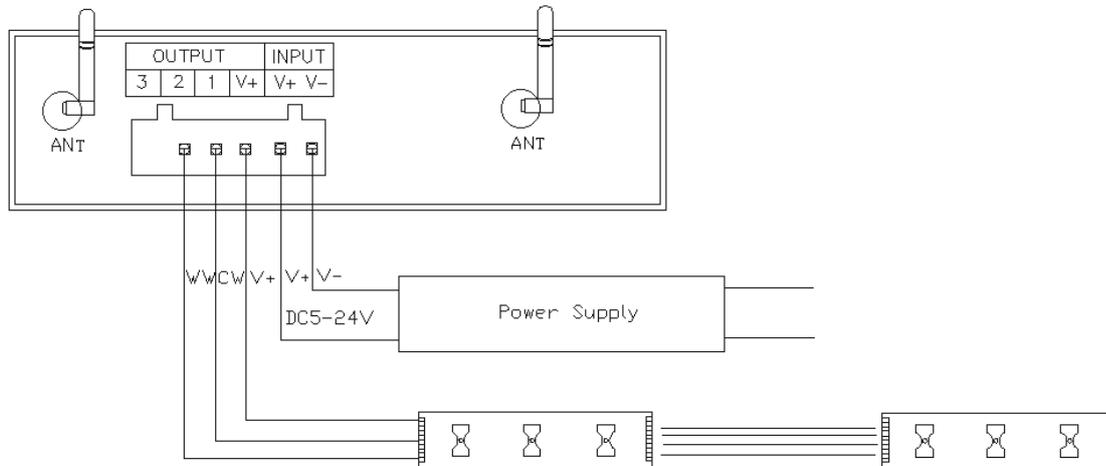
When connect three channels LED, you should put the Magic Color 1.0 software switch to CT mode to use, only under this mode, you can control the LED's color temperature, brightness and color temperature shortcut key settings. Color disk adjust the color temperature (meanwhile top left CW, WW numerical with change), brightness item adjust bright, "M" key set the special color temperature state.
