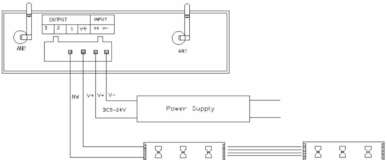
When connect three channels LED, you should put the Magic Color 1.0 software switch to DIM mode to use, under this mode, use color disk control the LED's brightness, Adjust process can be seen in the upper left corner NM numerical with change.
