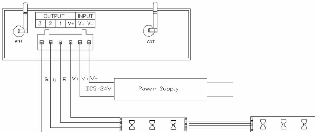
When connect three channels LED, you should put the Magic Color 1.0 software switch to CD mode to use, only under this mode, you can control the LED's color, brightness and speed. Color disk adjust the color (Adjust process can be seen in the upper left corner R, G, B numerical with change), speed/brightness item adjust speed and bright ("M" set the LED dynamic effect, "M" adjust the LED dynamic change).
